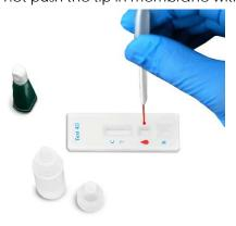
3. Add 2 full drops of Chase Buffer into the buffer well (Do not move the cassette after addition of buffer).
